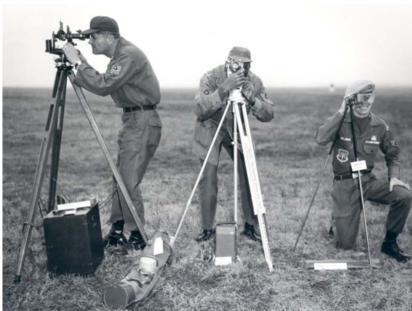
Theodolite and transit field test, ca. 1966-67. (l-r) Master Sergeants (unidentified) from the 5th Weather Wing are operating a standard theodolite (left) and Kern theodolite (center). SSgt Golding (right) is operating the Brunton Transit, later adopted for use with the effective wind system. (USAF photo)
