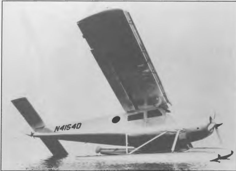
Putting the versatile U-10 on floats was an Air Commando innovation that had merit . . . as well as some obvious risks. Tested near Hurlburt Field, the idea was eventually dropped following the conclusion the latter outweighed the former. (ACA collection)
