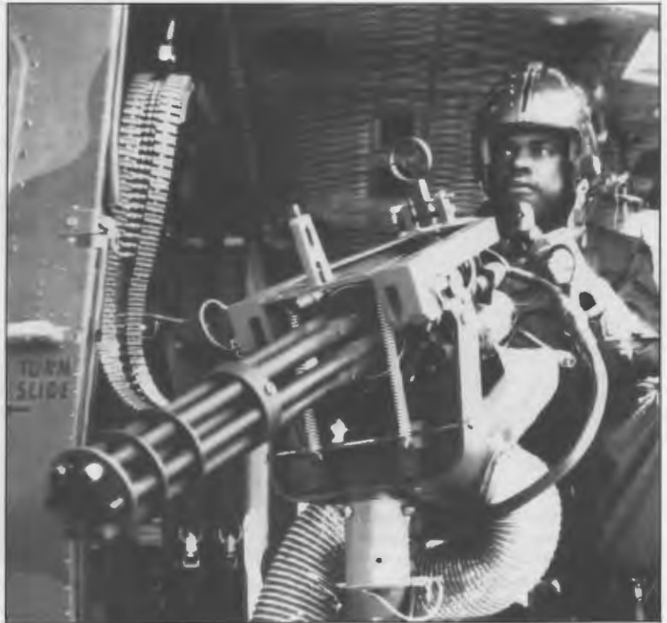
The 7.62mm minigun on a 20th SOS gunship could spit out 6,000 rounds per minute. This Green Hornet UH-1F helicopter is photographed on operations in South Vietnam, 1967. (USAF photo)
