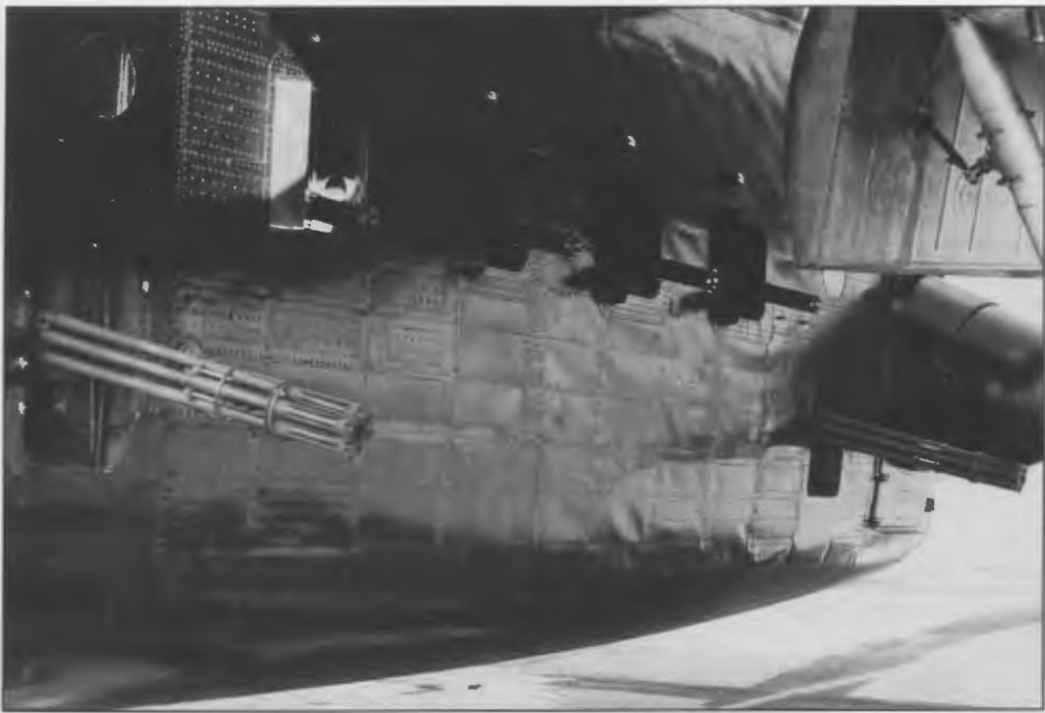
Like a fortress wall with its cannon, the lethal side of the AC-119K "Stinger" was just as deadly as it appeared. The 7.62mm miniguns were augmented with two additional 20mm cannon. The large weapons radar dome in the rear fuselage guided the firepower to target. (USAF photo)
