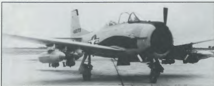
The T-28 fighter/bomber's simplicity and ruggedness made it an ideal strike aircraft for Water Pump students, some of which had never even driven a car until their arrival in Udon for flight training. Its two-seat configuration allowed for an interpreter or forward air controller if required, and its substantial munitions payload made it a weapon that could not be ignored by North Vietnamese and Pathet Lao troops. (ACA photo)
