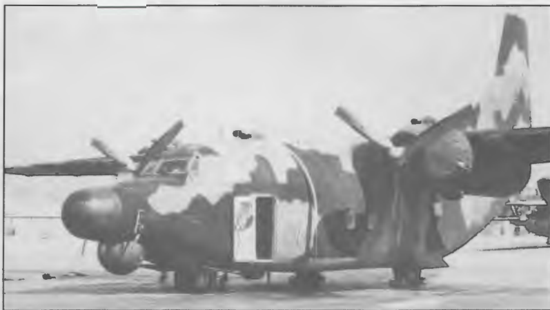
A rare photo of an even rarer aircraft, the NC-123K “Black Spot” bomber on pierced-steel-planking ramp at Ubon Royal Thai Air Base, February, 1969. This experimental concept called for the -123 to find targets with its own sensors, then bomb them. Mixed field results finally persuaded the Air Force to concentrate its efforts on the AC-130s of the 16th SOS. (John Ford, III)
