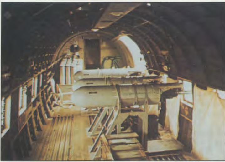
From inside "Puff the Magic Dragon", its three electrically-driven miniguns were impressive. Outside the gunship, these three guns firing together could put a bullet into every square yard of a football field in 3 seconds. (USAF photo)
