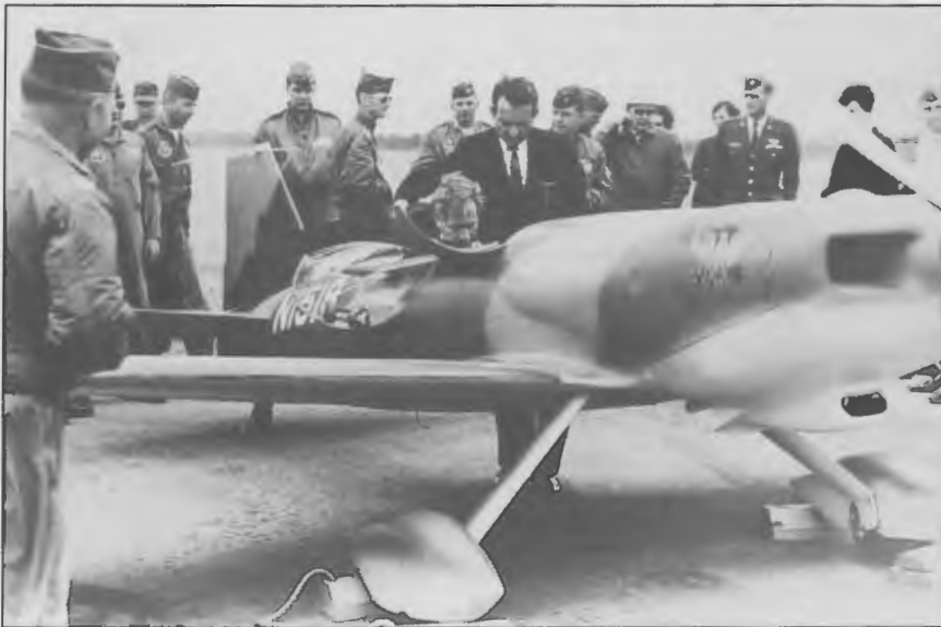
This experimental craft was built from the under-wing external fuel tank of a C-130 transport! Designed for low-level observation/strike missions, the idea was deemed impractical following testing. Note Air Commando emblem on fuselage. (ACA collection)
